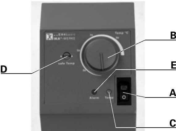
The EH4 basic suspended thermostat is turned on with the rocker switch (A). The „Temp“ rheostat dial (B) with accompanying temperature of the bath.
